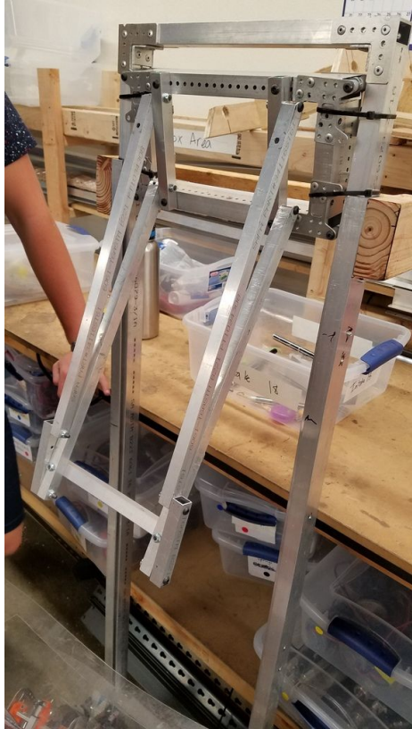
Prototype of cascading elevator and four bar arm
