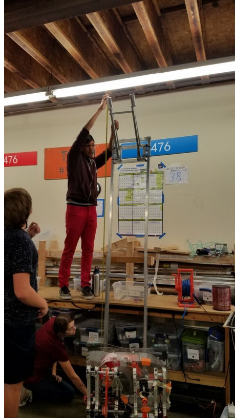
Prototype of cascading elevator and four bar arm
